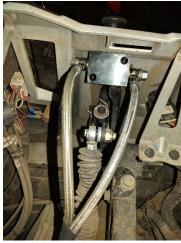
8. Remove tape on input brake line (line with banjo fitting only), DO NOT REMOVE tape on the exit line (with coupling). Remove rear brake line, banjo bolt, and both sealing washers from rear port of the master cylinder. Discard old sealing washers (never re-use sealing washers) and put a new washer on both sides of the input line banjo fitting and push removed banjo bolt through washers. Install bolt back into master cylinder and tighten to 15 lb-ft (20Nm).
