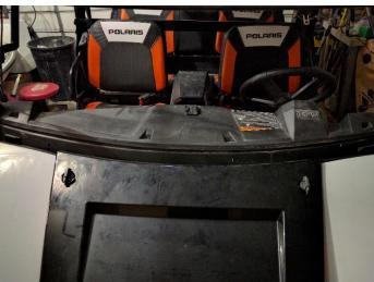
3. Cut out valve hole template and use packing tape to tape it to the installation location.
