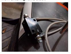
Route taped hose ends behind dash to brake master cylinder. DO NOT REMOVE TAPE YET. Reinstall valve body into valve block. DO NOT OVERTIGHTEN. Tighten valve body to 15 lb-ft (20Nm).
