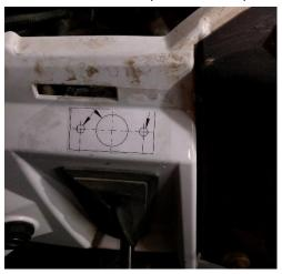
4. Drill both small holes first, then the large hole in the center.
